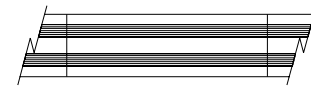
Option 13 Continuous Run Of Active And Inactive Sections For Hard Ceiling. Center "T"s Look Continuous With Options 11 Or 12 Separate Frame Around Perimeter.
