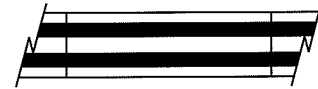
Option 13 Continuous Run Of Active And Inactive Sections For Hard Ceilings. Center "T"s Look Continuous With Options 11 Or 12 Separate Frame Around Perimeter.
